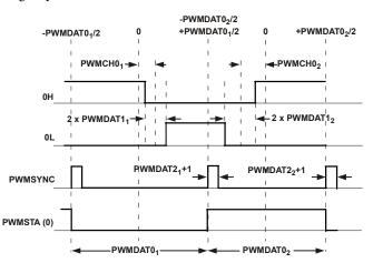
Figure 27: Typical PWM outputs of the Three-phase timing unit in double update mode
