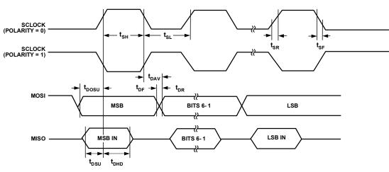
Figure 54. SPI Master Mode Timing (PHASE mode = 0)
