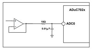
Figure 18: buffering single ended/pseudo differential input
