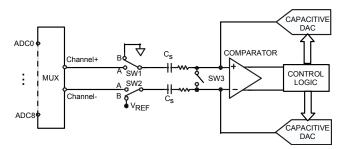
Figure 14: ADC conversion phase
