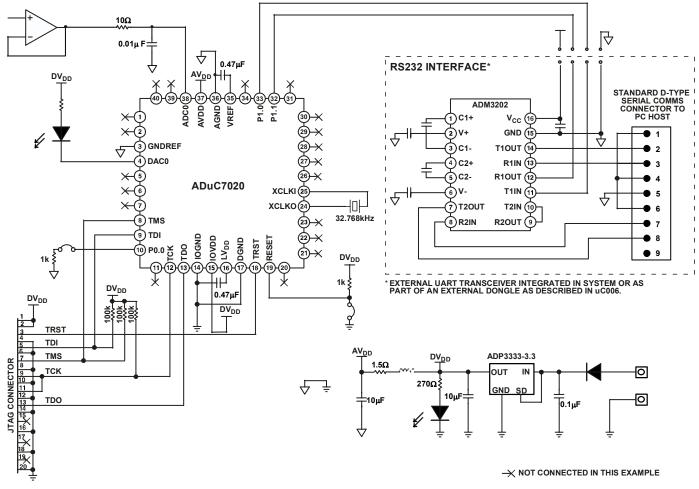
Figure 49:. Typical System Configuration
