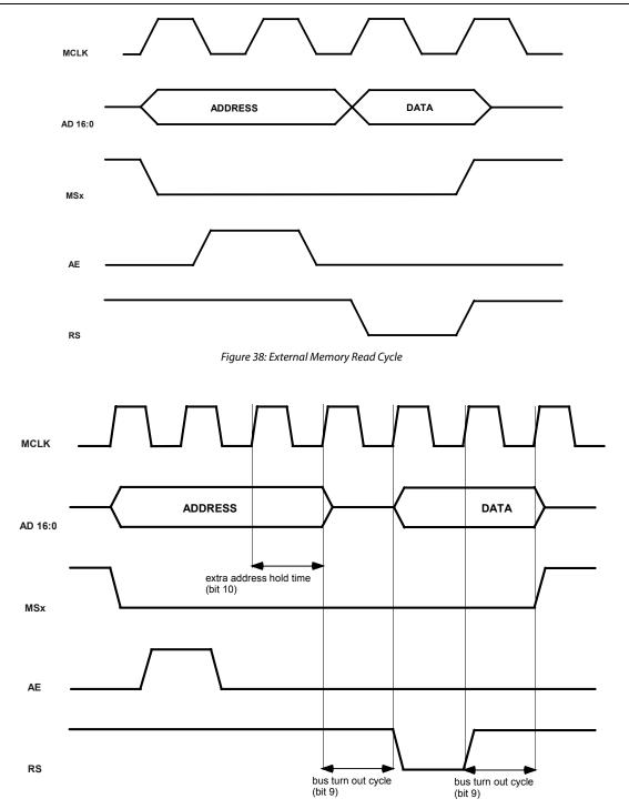
Figure 39: External Memory Read cycle with Address hold and Bus turn cycles
