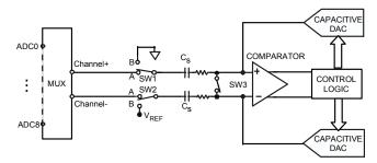
Figure 13: ADC acquisition phase
