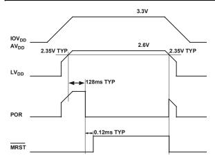
Figure 48: ADuC7024/ADuC7025 Internal Power-on-Reset operation
