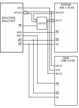
Figure 37 Interfacing to external EPROM/RAM
