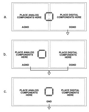
Figure 45:. System grounding schemes
