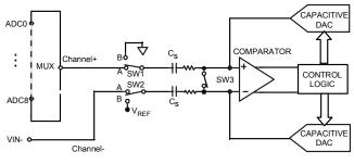
Figure 15: ADC in pseudo-differential mode
