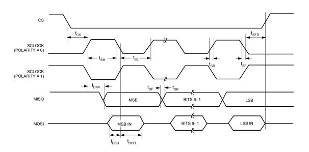
Figure 55. SPI Slave Mode Timing (PHASE mode = 1)
