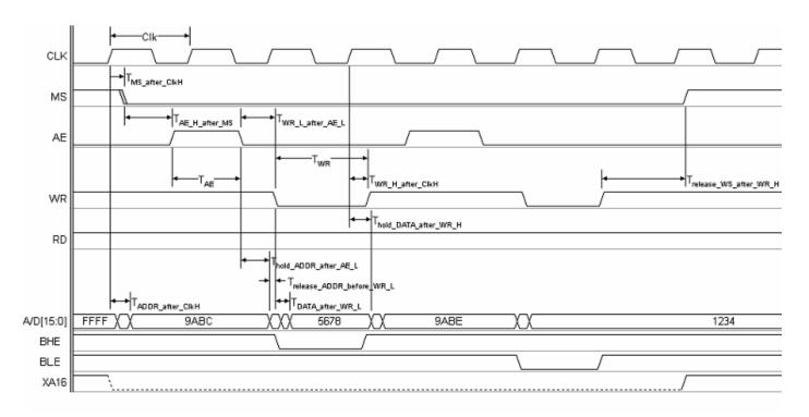
Figure 50: External Memory Write Cycle
