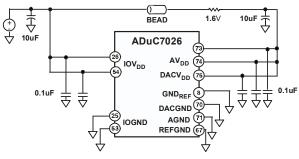
Figure 43: external single supply connections
