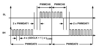
Figure 29: typical PWM signals with high frequency gate chopping enabled on both high-side and low-side switches
