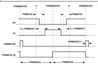
Figure 26: Typical PWM outputs of Three-Phase timing unit in single update mode
