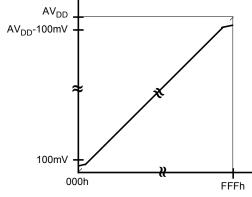
Figure 22: endpoint nonlinearities due to amplifier saturation
