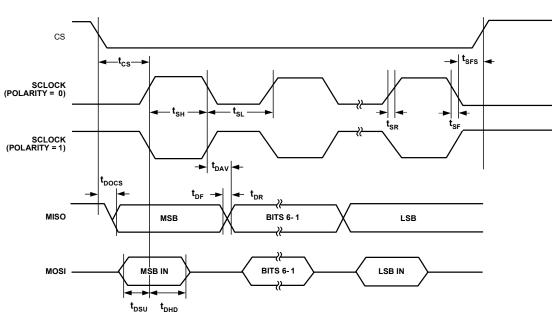
Figure 56. SPI Slave Mode Timing (PHASE mode = 0)
