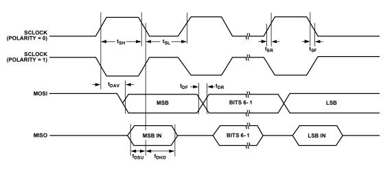
Figure 53. SPI Master Mode Timing (PHASE mode = 1)
