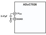
Figure 44: voltage regulator connections
