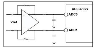
Figure 19: buffering differential inputs
