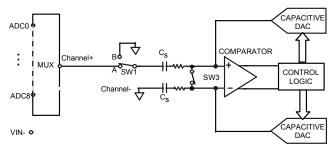
Figure 16: ADC in single-ended mode
