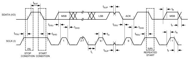
Figure 52: I<sup>2</sup>C compatible interface timing
