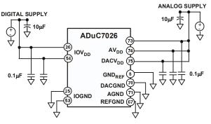
Figure 42: External dual supply connections
