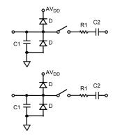
Figure 17: Equivalent Analog Input Circuit Conversion Phase: Switches Open Track Phase: Switches Closed
