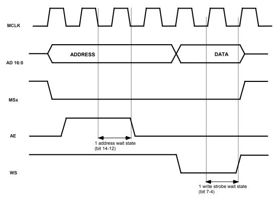
Figure 41: External Memory Write Cycle with wait states
