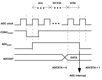
Figure 11: ADC Timing
