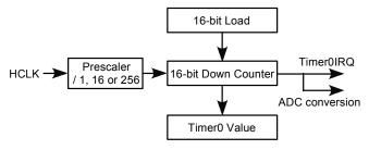
Figure 32: timer 0 block diagram
